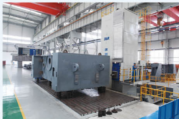
拥有数十台大型、重型数控机床和龙门式加工中心 Tens of large-scale heavy-duty CNC machine tools and gantry machining center
