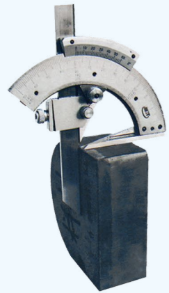
切割面垂直度检测 (板厚40mm) Verticality detection for cutsurface (thickness:40mm)
