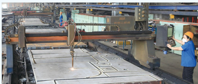
钢板下料均采用计算机自动优化排料和数控切割机切割 Steel plate blanking by means of computer automatic nesting and CNC cutting machine
